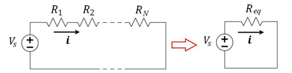
N resistors connected in series can be replaced by an equivalent resistor  $R_{eq}$
