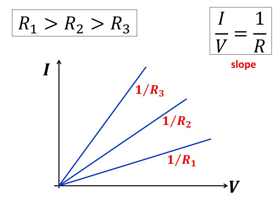
The smaller the slope, the higher the resistance
