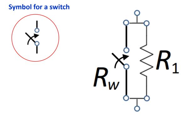
You can add a switch to turn on or off the effect of the shorting wire
