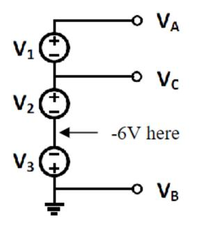
$$V_{A} = V_{1} + V_{2} - V_{3} = 9V$$
