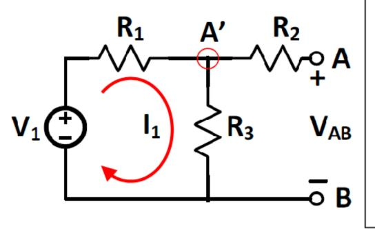
All points in the bottom wire are at the same potential as B. The circled node A' has the same potential as A, because no current flows in R<sub>2</sub>. The potential across R<sub>3</sub> is V<sub>AB</sub>. The only current flowing is I<sub>1</sub> through the series of R<sub>1</sub>+R<sub>3</sub>:
