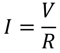
For low resistance *R*, a small voltage may cause a high current.
