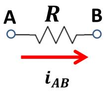
$$V_{AB} = i_{AB} \times R$$
