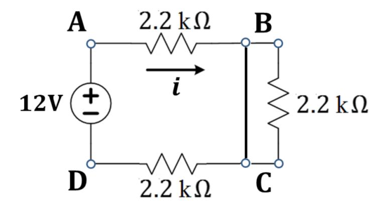
$i = 12/4,400 = 0.00\overline{27} \text{ A} = 2.\overline{72} \text{mA}$
