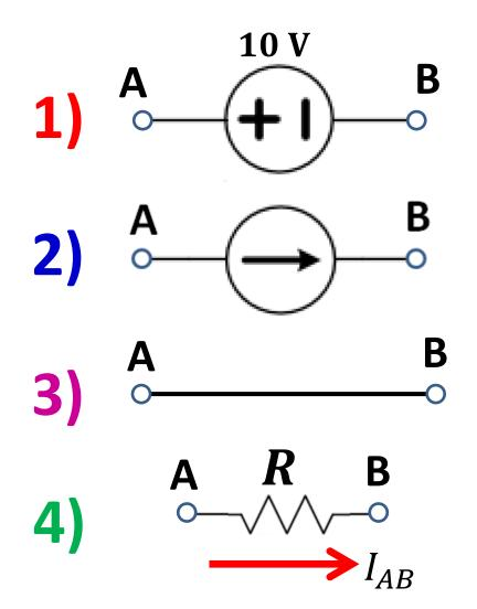
Ideal Voltage Source $V_{AB} = V_A - V_B$
