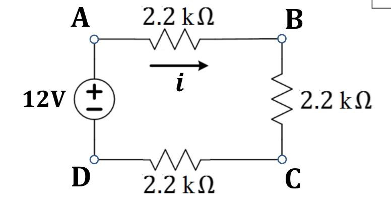
$R_{eq} = R_{AB} + R_{BC} + R_{CD} = 6.6 \text{ k}\Omega = 6,600\Omega$
