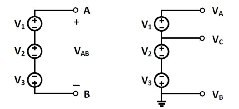
1. Compute voltage  $V_{AB}$ ,  $V_A$ ,  $V_B$ , and  $V_C$  in the circuits shown below. Assume  $V_1 = 10V$ ,  $V_2 = 5V$ , and  $V_3 = 6V$ .
