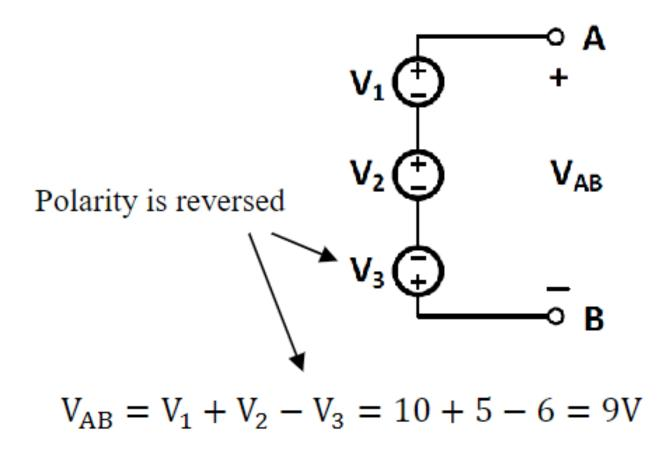
1. Compute voltage  $V_{AB}$ ,  $V_A$ ,  $V_B$ , and  $V_C$  in the circuits shown below. Assume  $V_1 = 10V$ ,  $V_2 = 5V$ , and  $V_3 = 6V$ .
