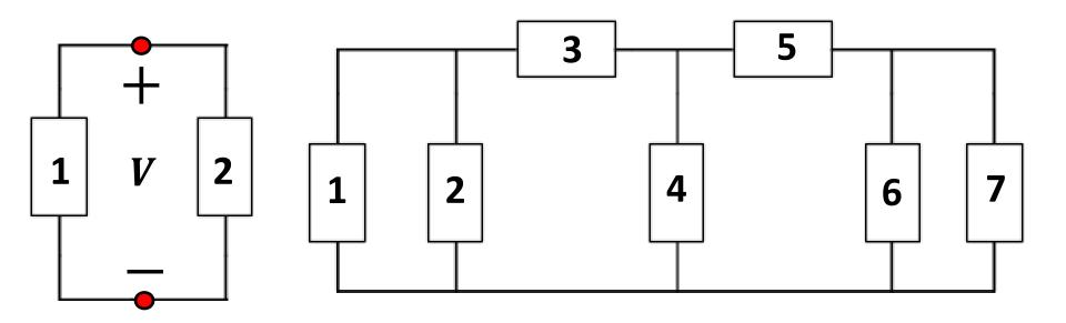
Which elements in the circuits above are connected in parallel?
