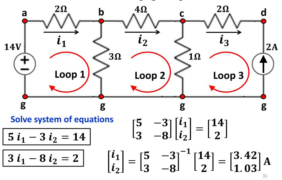
The simple system of equations can be solved by substitution
