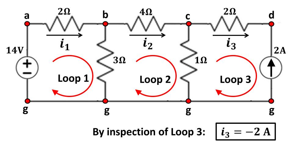
NOTE: Loop 3 has a current source. It is not possible to write a loop equation for it because the voltage  $V_{dg}$  depends on the rest of the circuit.
