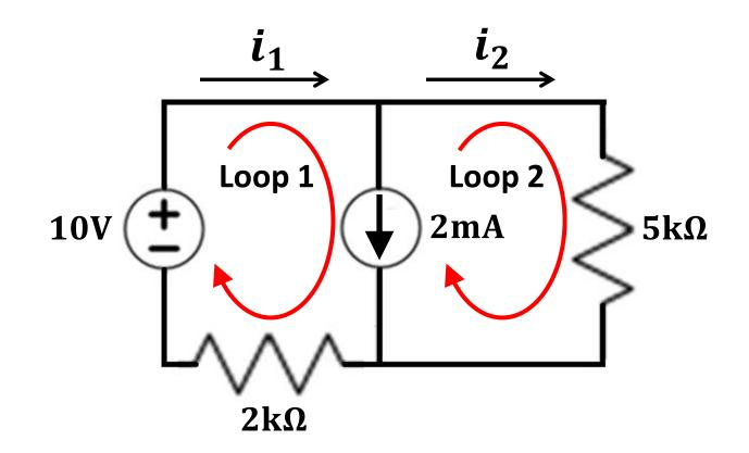
The two loops have a current source in the common branch and loop equations cannot be formulated.
