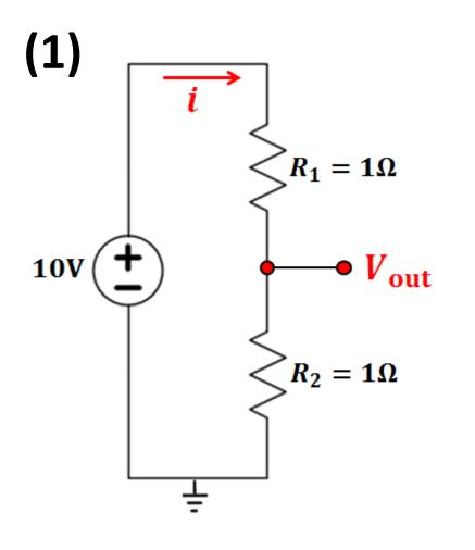
$$V_{out} = \frac{V_{in}R_2}{R_1 + R_2}$$
