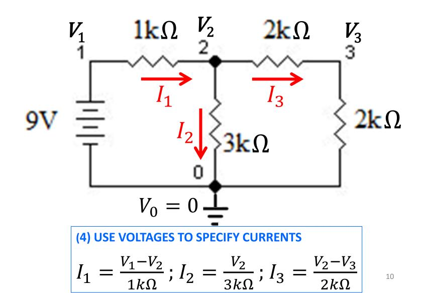
You could also define currents using indices between a specific node and neighboring ones <u>without specifying a fixed reference</u>. In this case it is good to write KCL with all outgoing currents.
