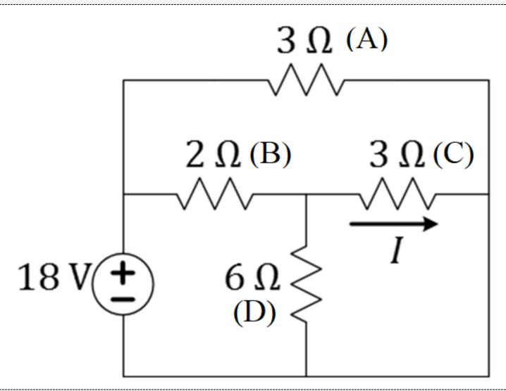
**Q:** Which resistor is in parallel with the voltage source?
