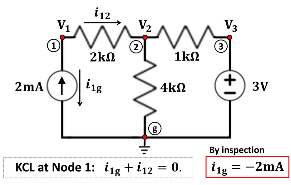
You may formulate the KCL equation in different equivalent ways, but it is good to have a consistent method.
