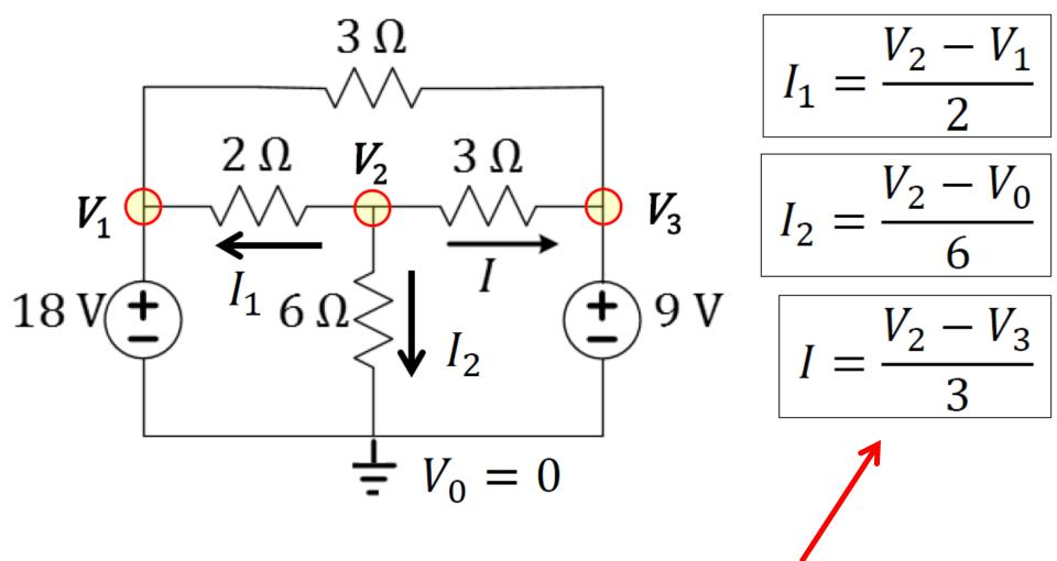
Now we should be comfortable with the method, so we can write the currents directly in terms of Amperes, without having to write all the time  $\Omega$ .
