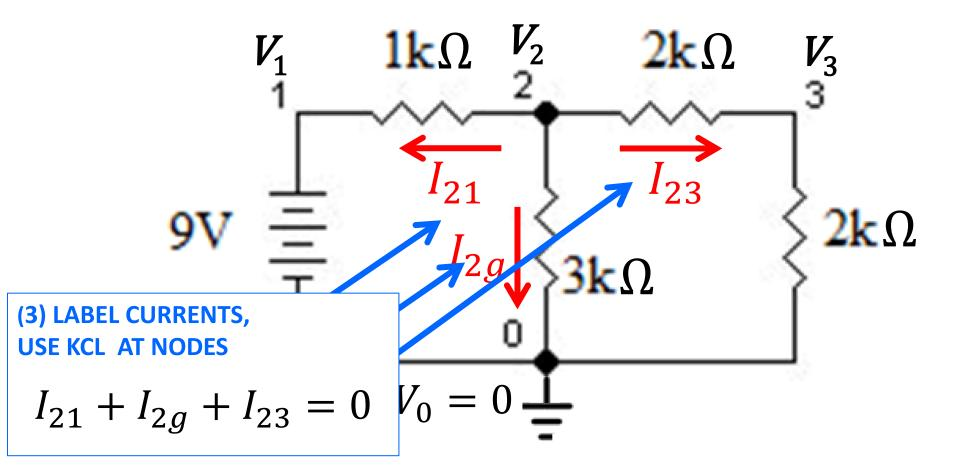
You could also define currents using indices between a specific node and neighboring ones <u>without specifying a fixed reference</u>. In this case it is good to write KCL with all outgoing currents.
