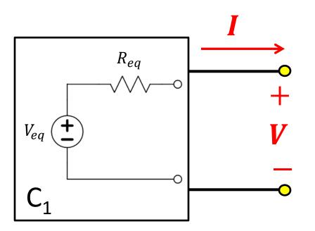
The equivalent source has the same terminal behavior of the original source sub-circuit
