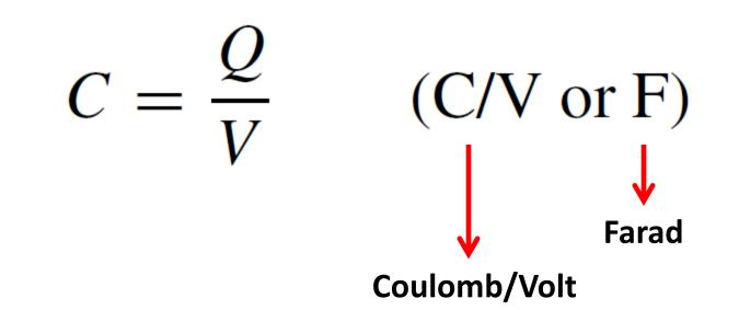
The capacitance *C* is independent of the electric field magnitude. It depends only on geometry (size, shape, positions) and on permittivity of the insulator (linear capacitor).
