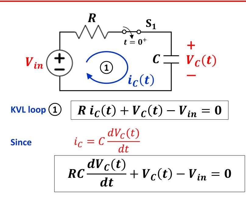
$$\frac{dV_C(t)}{dt} + \frac{(V_C(t) - V_{in})}{RC} = 0$$
