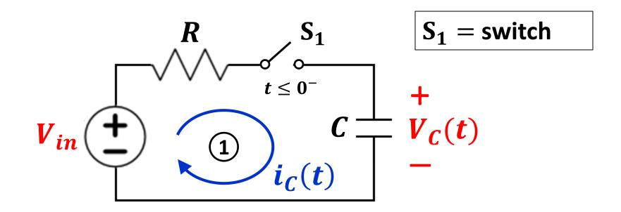
$V_{in}$  = constant voltage source (it does not change in time)
