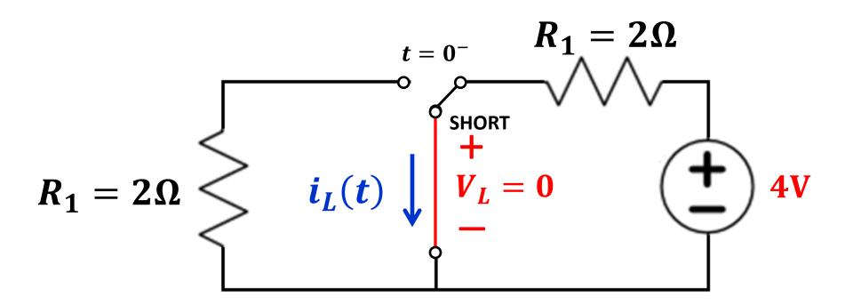
Step (1) Find  $i_L(0^-)$  and  $V_L(0^-)$  before the switch is closed
