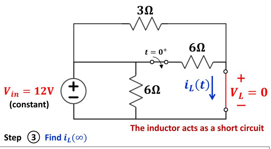
$$i_L(\infty) = K_2 = V_{in}/(3\Omega//6\Omega) = 12/2 = 6 \text{ A}$$
