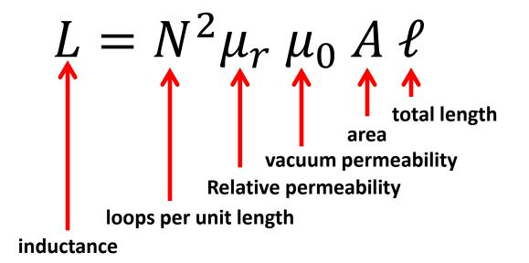
Example: Ferrite material used for compact antennas used in portable AM radios (medium wave frequency range)
