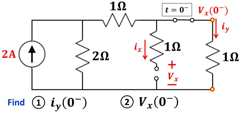
At  $t = 0^-$  the capacitor is an open circuit and  $i_{\chi}(0^-) = 0$ .
