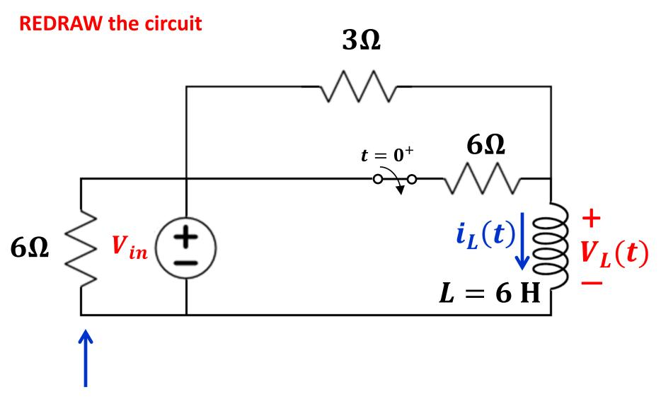
NOTE: This resistor does not affect the rest of the circuit because it is in parallel with the voltage source.
