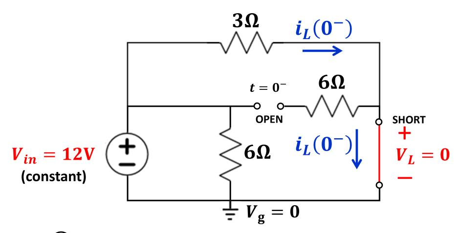
Step (1) Find  $i_L(0^-)$  and  $V_L(0^-)$  before the switch is closed
