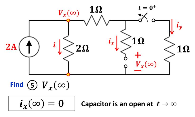
Capacitor has the same voltage as at the terminals of the  $2\Omega$  resistor through which flows the only current i = 2A
