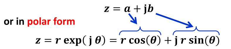
We wish to use complex functions to represent circuits driven by sinusoidal inputs at specific frequencies.
