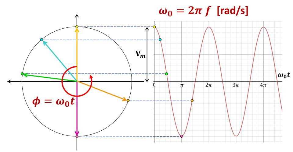
A vector with magnitude  $V_m$  and rotating at frequency  $\omega_0$  describes the evolution of a harmonic function on a 2D plane.
