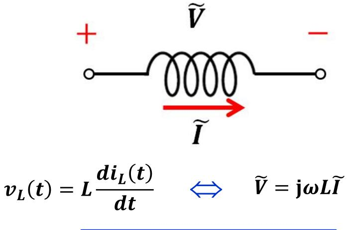
$$Z_L = \frac{\widetilde{V}}{\widetilde{I}} = \frac{V_m \angle \theta_v}{I_m \angle \theta_i} = \mathbf{j} \omega L$$
