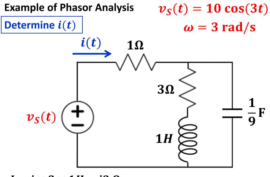
$j\omega L = j \times 3 \times 1H = j3 \Omega$  $1/j\omega C = -j/\omega C = -j/(3 \times 1/9 F) = -j3 \Omega$
