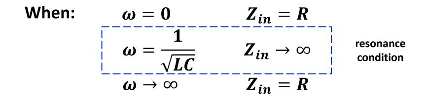
At the resonance condition, the reactance (parallel of *L* and *C*) behaves like an open circuit and no current can flow.
