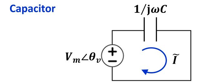
$$\widetilde{I} = \frac{V_m \angle \theta_v}{\frac{1}{j\omega C}} = j\omega C V_m \angle \theta_v = \omega C V_m \angle (\theta_v + \pi/2)$$
