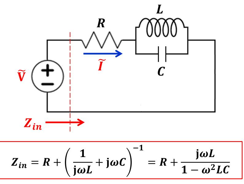
$$Z_{in} = R + \left(\frac{1}{j\omega L} + j\omega C\right)^{-1} = R + \frac{j\omega L}{1 - \omega^2 LC}$$
