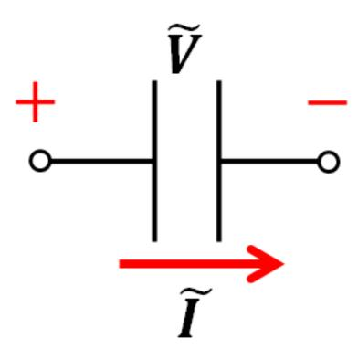
$$Z_{C} = \frac{\widetilde{V}}{\widetilde{I}} = \frac{V_{m} \angle \theta_{v}}{I_{m} \angle \theta_{i}} = \frac{1}{j\omega C} = -j\frac{1}{\omega C}$$
