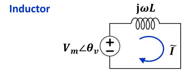
$$\widetilde{I} = \frac{V_m \angle \theta_v}{j\omega L} = -j \frac{V_m \angle \theta_v}{\omega L} = \frac{V_m}{\omega L} \angle (\theta_v - \pi/2)$$
