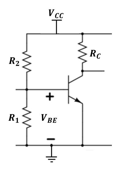
$$R_{eff} = R_1 / / R_2$$
