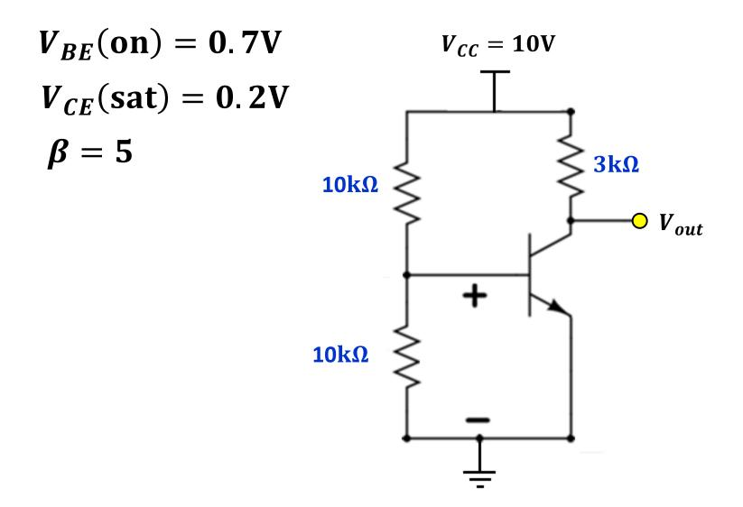
$$R_{eff} = R_1 / / R_2 = 5k\Omega \qquad V_T = 10 \frac{10k\Omega}{10k\Omega + 10k\Omega} = 5V$$
