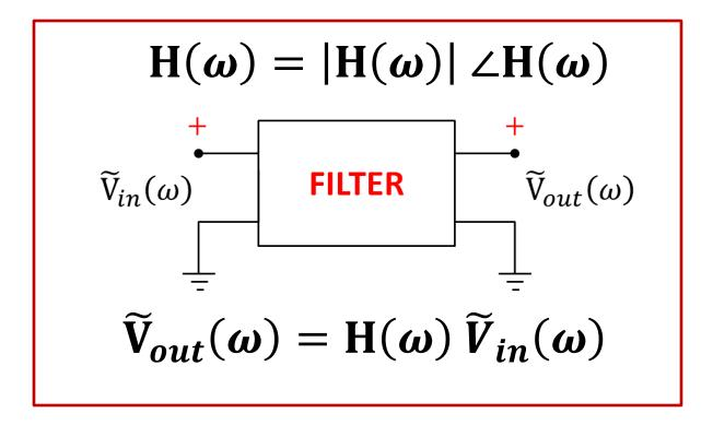
$V_{out}(t) = |\mathbf{H}(\boldsymbol{\omega})|V_{\mathbf{m}}\cos(\boldsymbol{\omega}t + \boldsymbol{\theta}_{V} + \angle \mathbf{H}(\boldsymbol{\omega}))$
