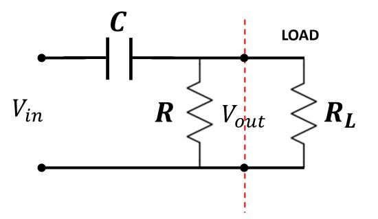
The parallel  $R_{eff} = R//R_L$  yields an equivalent resistance lower than either R or  $R_L$ . In particular, if connected to a small resistor  $R_L$ , the resulting cutoff frequency  $\omega'_C = (R_{eff}C)^{-1}$  may change considerably with respect to the original  $\omega_C = (RC)^{-1}$ .
