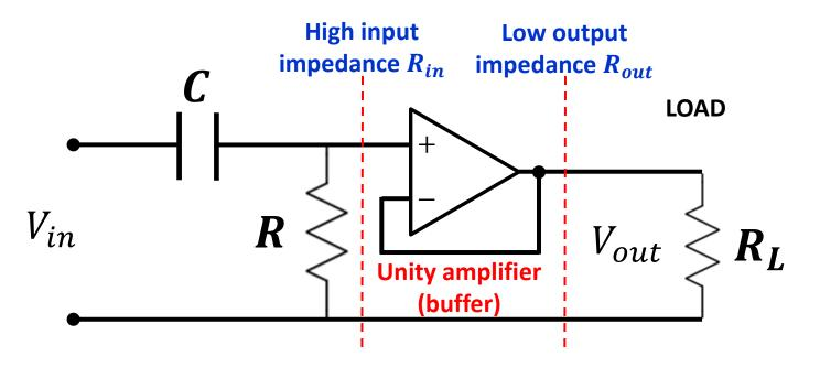
The filter sees  $R//R_{in} \approx R$  and is not affected. In output the voltage  $V_{out}$  drives a total resistance  $R_{in} + R_L$ . If  $R_{out}$  is much smaller, power is delivered mainly to the load  $R_L$ .
