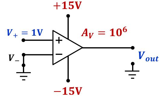
$$V_{out} = A_V \times (V_+ - V_-) = 10^6 (1 - 0) = 10^6 V$$
