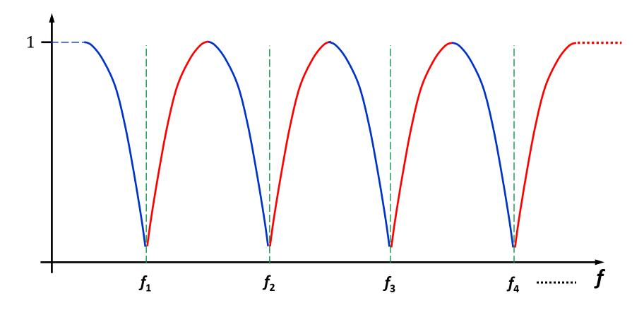
The comb filter consists of a series of regularly spaced notches and peaks (also called *teeth*).
