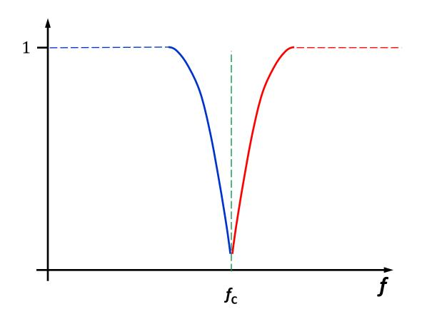
A very narrow band-stop filter, designed to reject a specific frequency, is called a notch filter.
