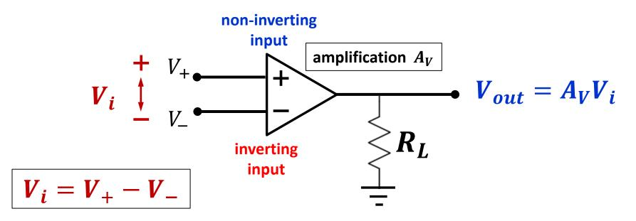
The gain between  $V_{out}$  and  $V_+$  is positive (non-inverting)
