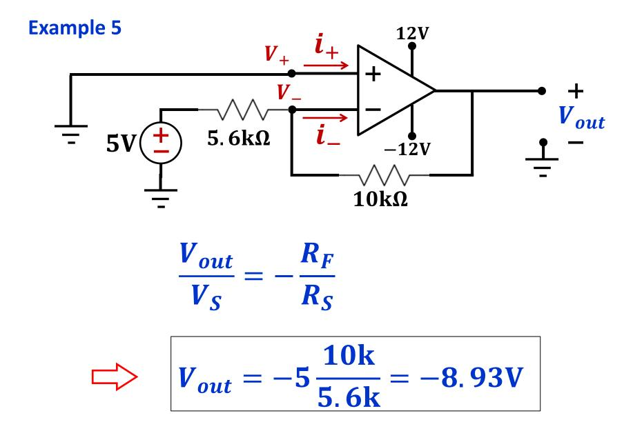
Since  $|V_{out}| < |V_{CC}|$ , the result obtained is valid.
