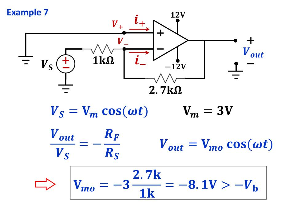
Since  $|V_{mo}| < |V_{CC}|$ , the result obtained is valid.
