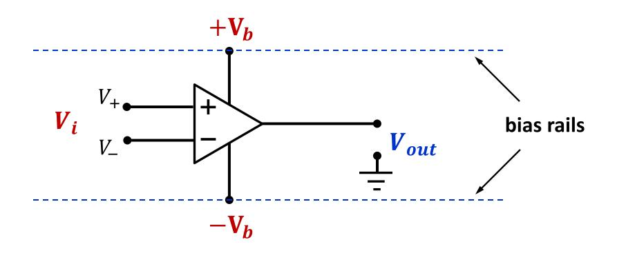
The output signal  $V_{out}$  can swing between  $\pm V_b$  but it will saturate if trying to exceed  $|V_b|$ .
