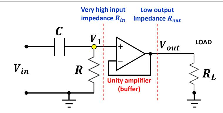
$V_{out} = V_1$
