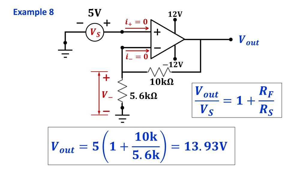
Since  $|V_{mo}| > |V_{CC}|$ , the op-amp saturates at 12V. In Example 5, with the same resistors the inverting op-amp did not saturate.
