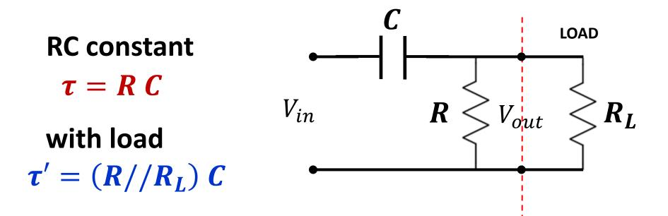
The parallel  $R_{eff} = R//R_L$  yields an equivalent resistance lower than either R or  $R_L$ . In particular, if connected to a small resistor  $R_L$ , the resulting cutoff frequency  $\omega'_C = (R_{eff}C)^{-1}$  may change considerably with respect to the original  $\omega_C = (RC)^{-1}$ .
