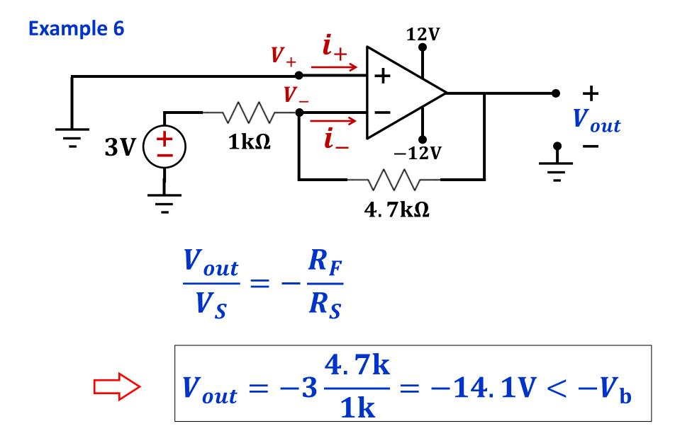
Since  $|V_{out}| > |V_{CC}|$ , the output voltage saturates at  $-12V_{24}$
